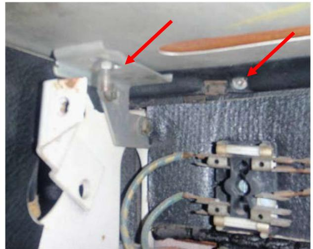
Inside the center instrument panel and underneath the dashboard. This view is of the left side. Note 5/16" retaining nut on vertical screw and Phillips head screw at upper rear. The right side is identical. All four must be removed in order to lift out the dashboard.
