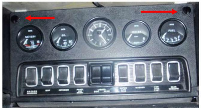
The thumb screws are in the upper corners of the center instrument panel.
